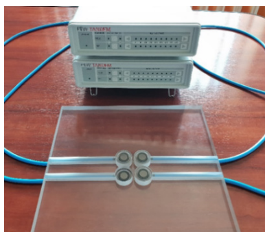
Fig. 1 The first demonstrative prototype of the QADRO-fm detector, with the dual channel electrometers for readout.
